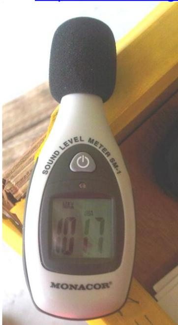
Over a period of more than twelve months we recorded background noise on numerous different car carriers, at different ports in a number of different countries, and we found that these noise levels could easily surpass 80db and peak levels often exceeded 100 db.
